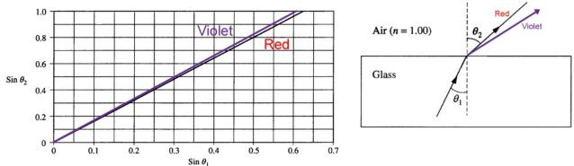
a. Assuming an index of refraction of 1.00 for air, use the graph to determine a value for the index of refraction of the glass for the red light. Explain how you obtained this value. For this red light, determine the following.
